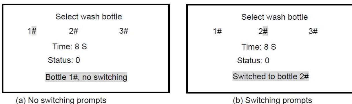
Fig. 3-9 Switching the wash bottles
